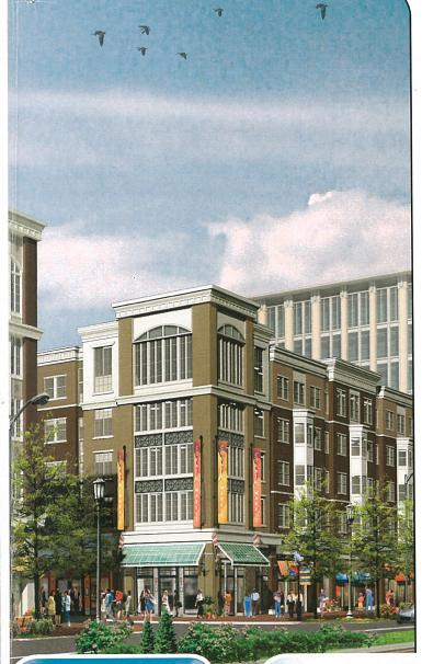
Using the IBC construction Type Va (5a) R-2 over Type la (1a) M retail space or S-2 garage will restrict the height to five stories (4 over 1) and 70', allowing the two stacked buildings to be designed somewhat separately with unique fireproofing and waterproofing conditions. This construction type is fairly new to the east coast and mid-west so additional approval effort may be necessary. This building type is rarely found outside of urban or new-urban town center environments.
